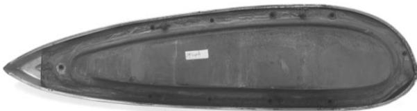
4. Next remove the lens to gain access to the housing. There are ten (10) screws that hold the lens in place, remove the screws and separate the lens carefully.
