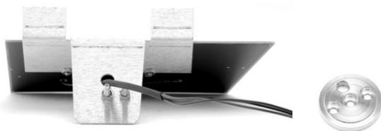
6. Pass the wires through the housing where the original bulb and socket were. Set the LED assemblies into the housing so the studs extend out the hole in the bottom of the housing.
