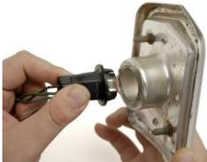
2. Remove the tail light housing hardware so the housing can be removed from the car. Remove the housings from the vehicle carefully so the body gaskets are not damaged.
