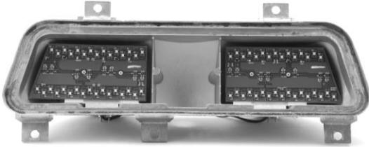
7. Feed the wires through the larger hole in the mounting plate. Guide the mounting plate to the bottom of the housing. The flat side of the mounting plate should be down and the side with the slight raised center should go up toward the housing. This will align the mount in the original housing.
