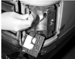
8. After the primer has had adequate time to dry, remove the backing from the tape located on the LED assembly.
