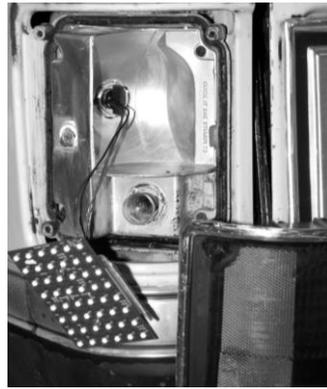
7. Make sure the tail light housings are clean and dry so the single use primer applicator can be used for both housings. Apply the primer to the outside edge of the housing where the tape will attach. **AFTER THE PRIMER HAS BEEN APPLIED, LET THE HOUSING DRY FOR 5 MINUTES BEFORE GOING ON.**
