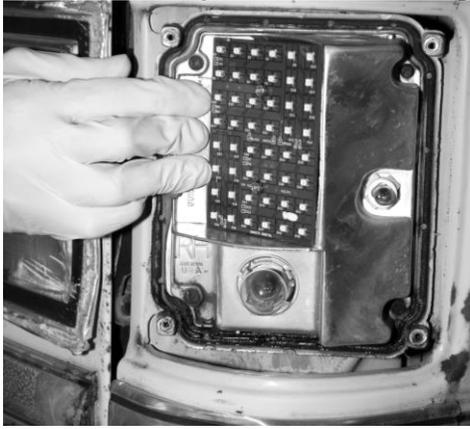
10. Fasten the lens back on with the four original screws.
