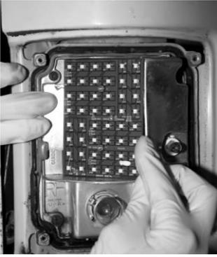
6. Before mounting the new LED assembly into the housing, plug the bulb base into the stock bulb socket and test the tail lights and flashers to make sure everything is working correctly.
