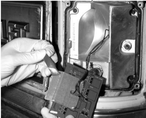
9. Make sure the bulb base is fastened securely in the stock bulb socket. Carefully place the LED assembly onto the housing and press down firmly.
