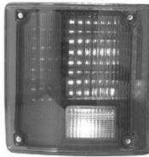
1. Remove the tail light lenses. There are four screws holding each lens in place.
