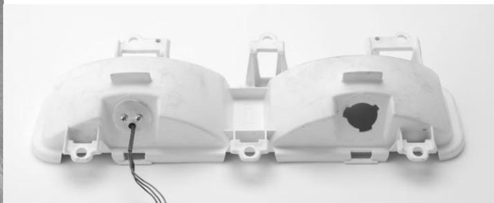
8. Install the lens and/or re-assemble the tail light housing, insuring all gaskets are intact and in place. Install the tail light housing back into the vehicle. You are now ready to wire the LED assembly into the vehicle tail light harness.
