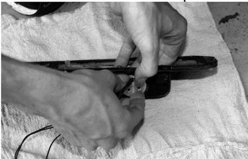
7. Screw the mounting plate into the assembly mount using the two previously removed 3/8" 6-32 screws.
