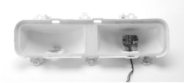
Feed the wires through the larger hole in the mounting plate. Guide the mounting plate to the bottom of the housing. The flat side of the mounting plate should be down and the side with the slight raised center should go up into the housing. This will align the mount in the original housing.
