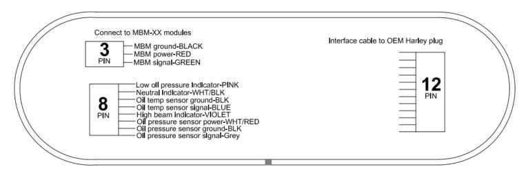
The interface harness allows the stock H-D data bus harness to adapt to the MLX-9x04
