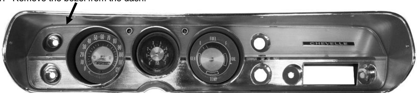
2. Remove the stock gauge, and lens from the bezel. The only item to be reused is the original front bezel.
