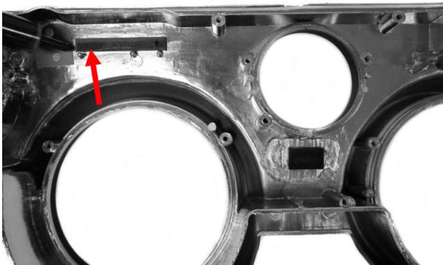
4. The stock indicator for Brake will not be used. Use the included block-off plate which has "636109" engraved on it. RTV silicone works well to secure these plates. Be sure to glue it with the textured side down to ensure the part numbers are not visible from the front side.
