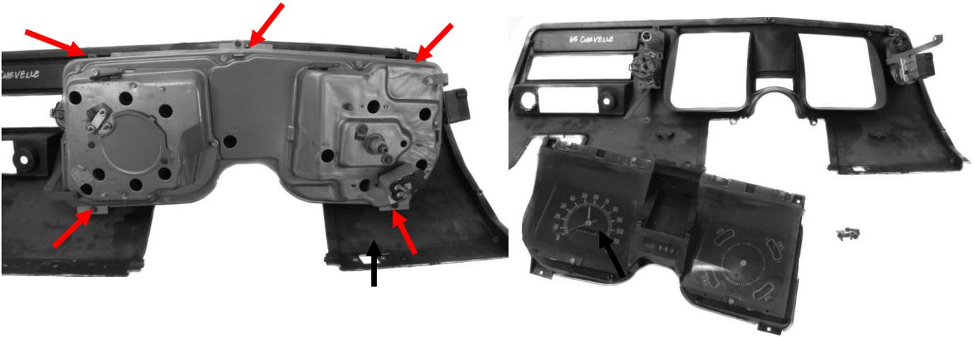
3. Remove the seven screws that hold the stock gauges to the lens spacer. Save this hardware as it will be reused.
