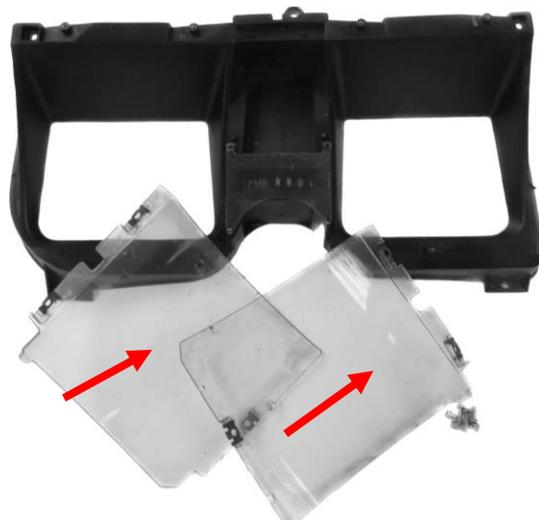
5. The stock gear-position indicator (automatic bezels only) will be eliminated with the installation of the RTX system. A black-out plate is supplied and can be glued in place of the stock indicator. If you purchased a separate GSS-3000 kit from Dakota Digital, the gear position can be displayed in the RTX message centers; therefore the stock gear position indicator can be removed.
