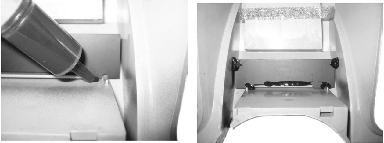
6. Install the RTX system into the stock lens spacer by securing the system to the spacer by reusing the seven screws removed in step 3.
