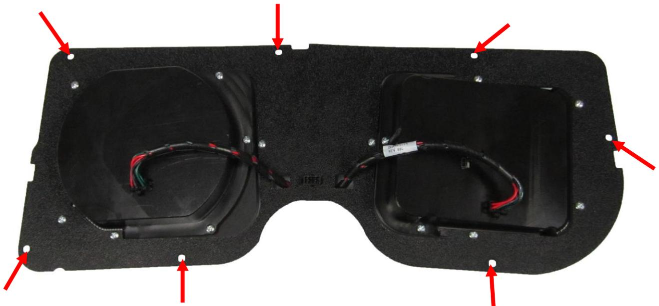
7. Connect the provided Main Harness and the Buzzer (optional for audio feedback) to the back of the RTX system.
