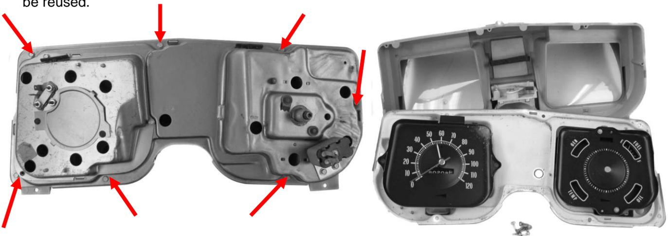
4. Remove the stock lenses from the lens spacer by removing three screws from the front of each lens. The stock lenses are removed since the new RTX kit features hard coated clear lenses.
