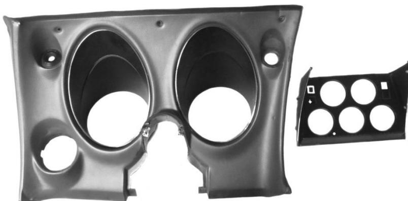
2. Remove the stock gauges, separator plate, and lenses from the bezels. For the main cluster, reattach the lens spacer to the bezel after removing the lens as shown. The only items to be reused are the original front bezels and gauge mounting hardware.
