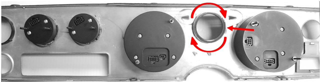
6. Slide the rear main housing over the speed and tach gauges and fasten into place using the provided thumb nuts. Then use the provided cups, leveling bracket and thumb nuts to secure the two satellite gauges in place.
