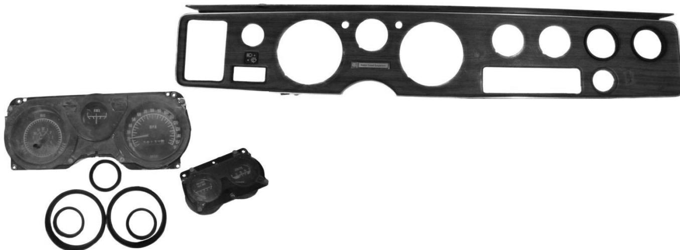
3. Remove the four thumb nuts from the back of the main housing, then remove the rear main housing from the speed and tach gauges.
