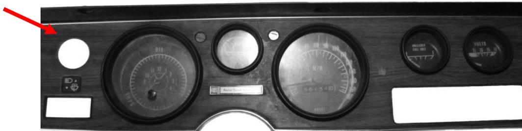
2. Remove the stock gauges and trim rings from the bezel. These items will not be reused and can be set aside.
