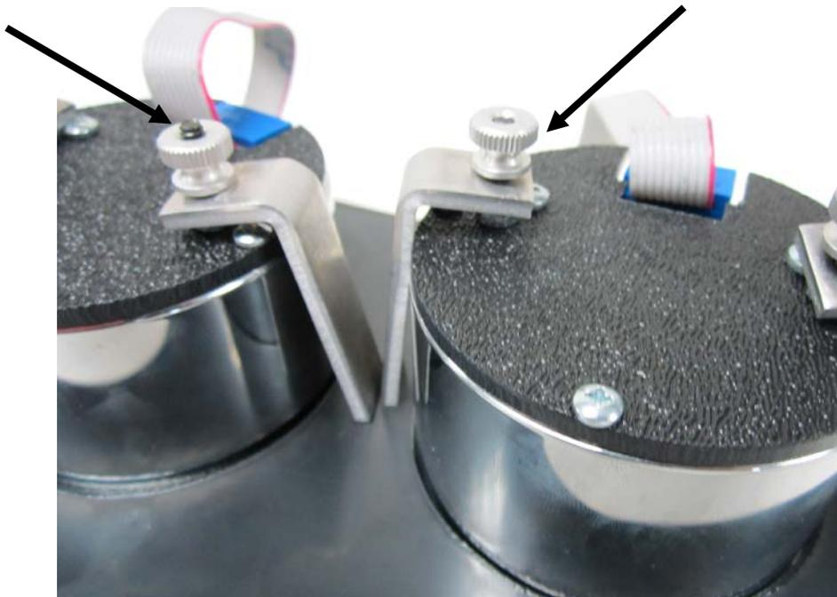
3. Make the proper connections between the four (4) labeled ribbon cables from the main gauge to the lead from each small gauge. Example; Fuel cable from the main gauge connects to the Fuel auxiliary gauge cable.
