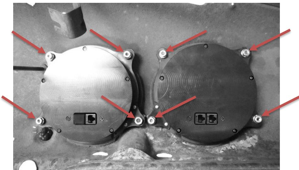
5. Connect the two halves of the new VHX system with the supplied 12" CAT5 cable. Also, route the 36" cable towards the control box location and connect it to the display.
