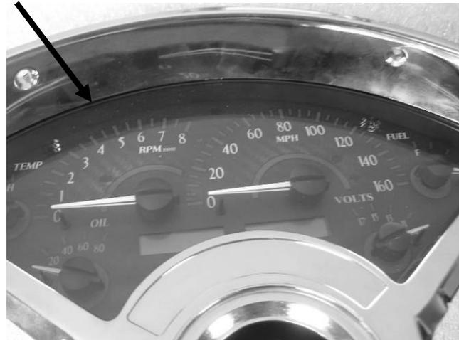
9. Secure the VHX system to the bezel with the six 8-32 x 1.25" screws and lock washers provided.
