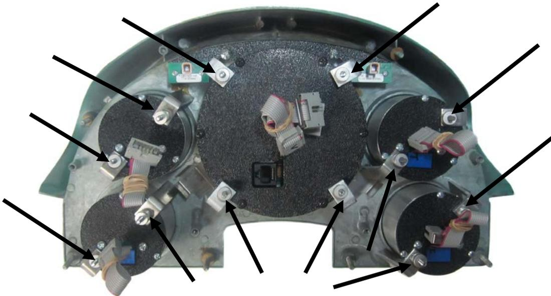
4. Make the proper connections between the four (4) labeled ribbon cables from the main gauge to the lead from each small gauge. Example; Fuel cable from the main gauge connects to the Fuel auxiliary gauge cable.
