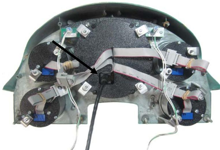
7. Re-install the gauge cluster to the dash using the factory hardware and refer to the main manual for wiring instructions to complete the VHX installation.
