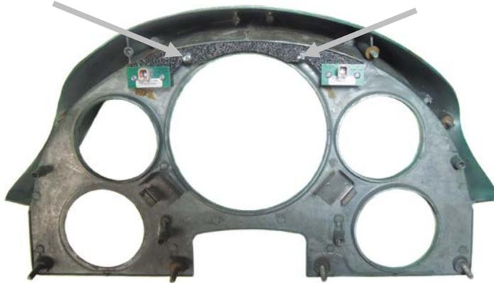
3. From the front, place the main gauge and the four small gauges through the bezel in the stock locations or arrangement of your choice; secure the gauges to the bezel by using the provided L-Brackets and thumb nuts. NOTE: the four (4) longer L-Brackets are used for the large main gauge.
