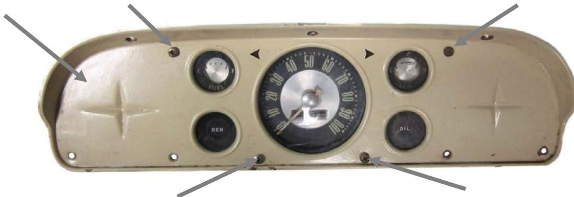
2. Secure the VHX system to the gauge panel using the four screws from disassembly.
