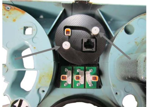
8. Remove the lens from the two large bezels and reuse the same screws to mount the bezels to the VHX speed and tach displays.
