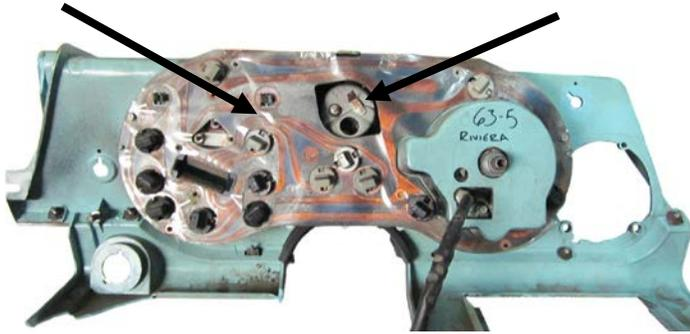
2. Remove the clock and all the gauge parts on the back of the gauge panel.
