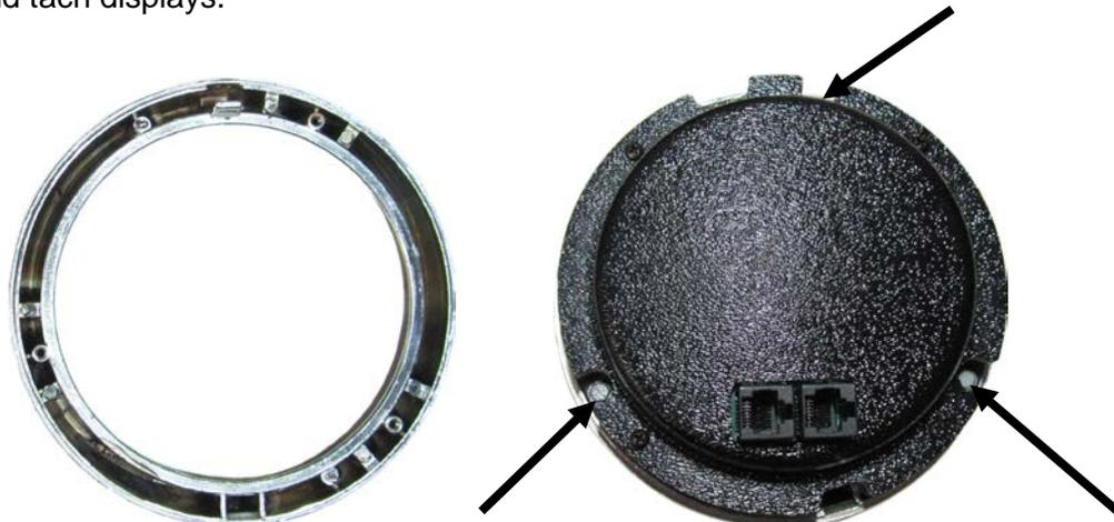
9. With the bezels attached, place the VHX speed into the left opening and the VHX tach into the right. Ensure there are no obstructions with fitment, if there is review step 5. With proper fitment use the two set crews from disassembly and secure the bezels to the housing.
