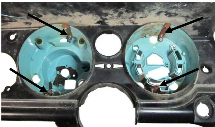
4. The bezel mounting tabs will be reused and can remain in place; all other pieces need to be removed and set aside.
