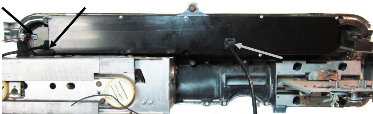
6. The cluster is now ready to re-install into the vehicle using stock hardware, take care when routing the CAT5 cables to the control box mounting location. Refer to the main manual and the 650462 clock manual for wiring instructions to complete the VHX installation.
