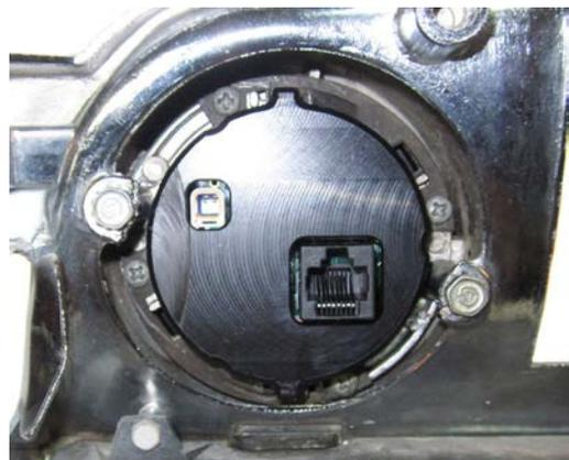
5. Mount the VHX System to the stock bezel using the same hardware from disassembly. Connect the 36" CAT5 cable to the back of the VHX system while the 60" CAT5 cable will connect to the clock as well as the clock power harness.
