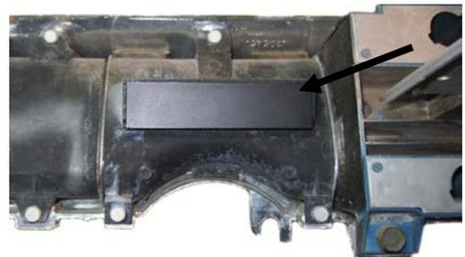
4. Secure the VLC Clock by placing it into the clock bezel opening from the front orientated as shown below; rotate the clock in a counter-clockwise direction until the mounting tabs lock into place.
