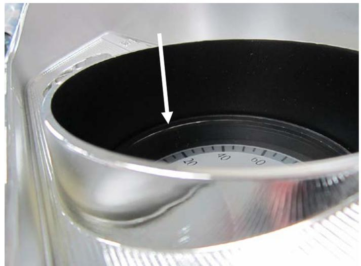
4. Secure the VHX system to the bezel using the four 8-18 x 3/4" screws.
