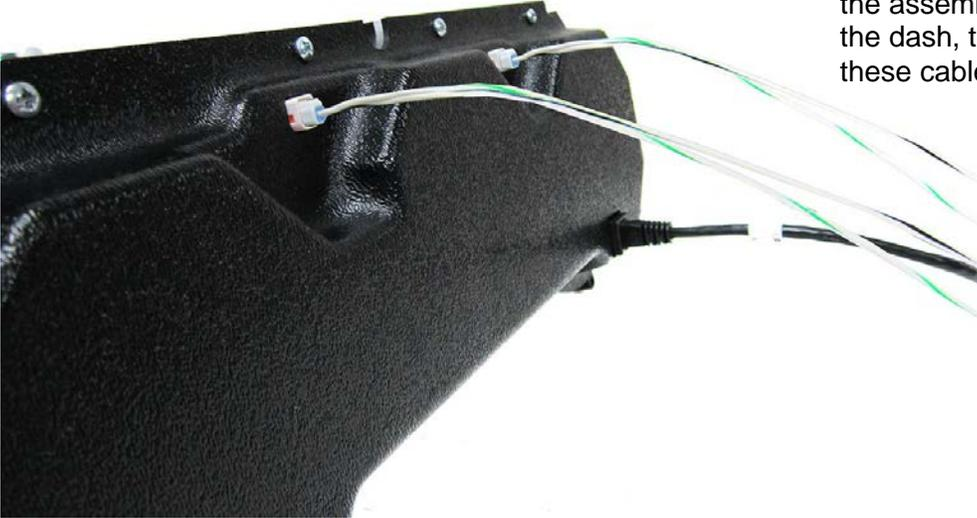
7. Re-install the cluster into the dash and refer to the main manual for wiring instructions to complete the VHX installation.
