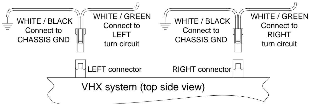
6. Connect the CAT5 cable and the two blinker harnesses to the system. As the assembled cluster is installed into the dash, take care when routing these cables to the control box.
