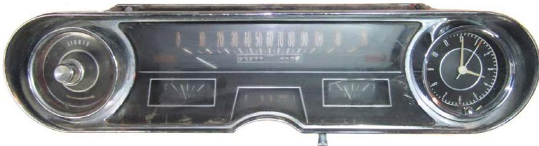
2. Looking at the back of the gauge cluster; remove the clock, speedometer, headlight switch assembly, and mounting brackets so you are left with a bare bezel. Use a 5/64 allen wrench for the set screw at the bottom of the bezel to remove the clock and headlight assembly.
