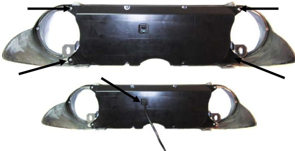
4. Mount the bezel assembly to the dash using the same hardware from disassembly. Take care when routing the CAT5 cable to the control box mounting location.
