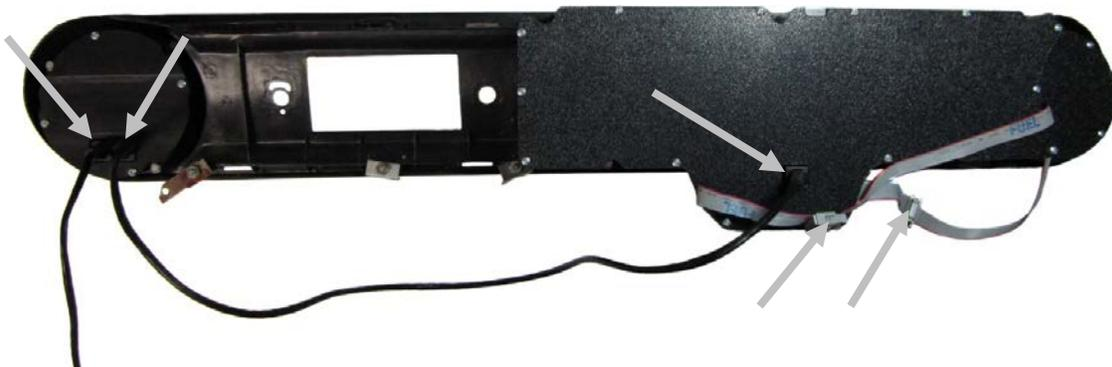
5. If you decide to not use the factory clear lens you can use the supplied trim pieces to cover the openings where the factory lens snapped into place. Simply peel off the front scratch resistant covering and the backing to expose the adhesive, line up and center the longer piece for the bottom and the shorter piece for the top.
