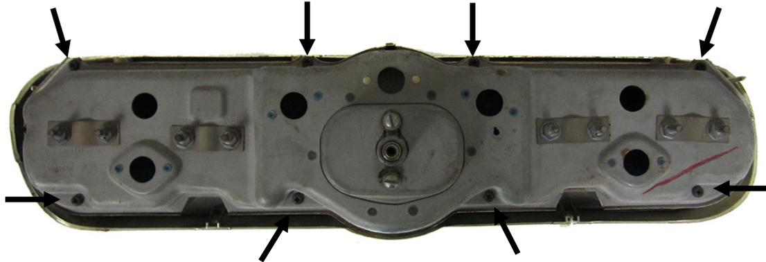
2. Remove the stock gauges and lens from the bezel. The only items to be reused are the original front bezel and four (4) of the stock mounting screws; the other pieces can be discarded. Now is a good time to clean the bezel or upgrade to a new one.
