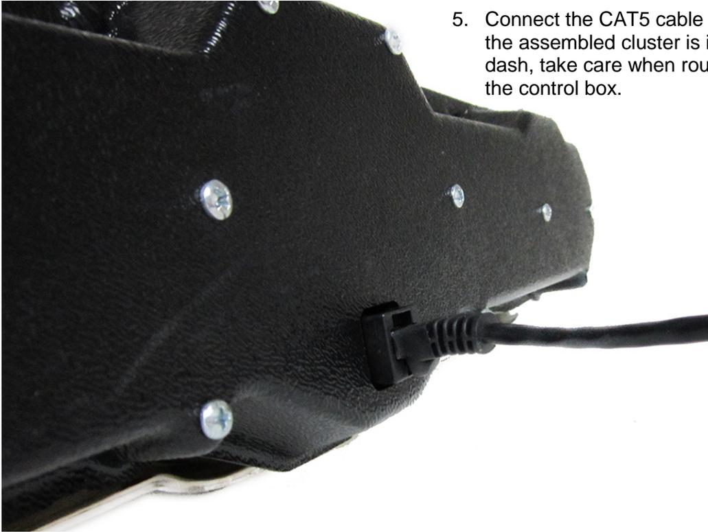
5. Connect the CAT5 cable to the system. As the assembled cluster is installed into the dash, take care when routing this cable to the control box.
