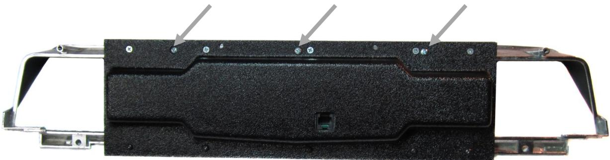
8. Attach the assembled gauge trim to gauge housing using five (5) 6-20 X 5/8" screws.
