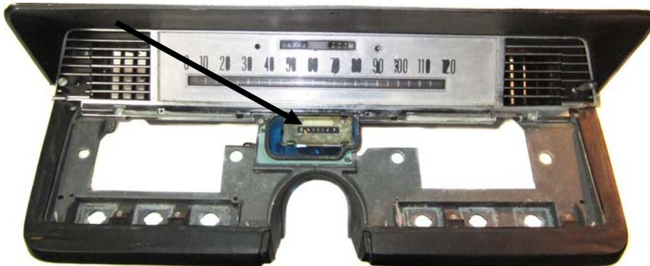
4. Remove the speedometer gauge face.
