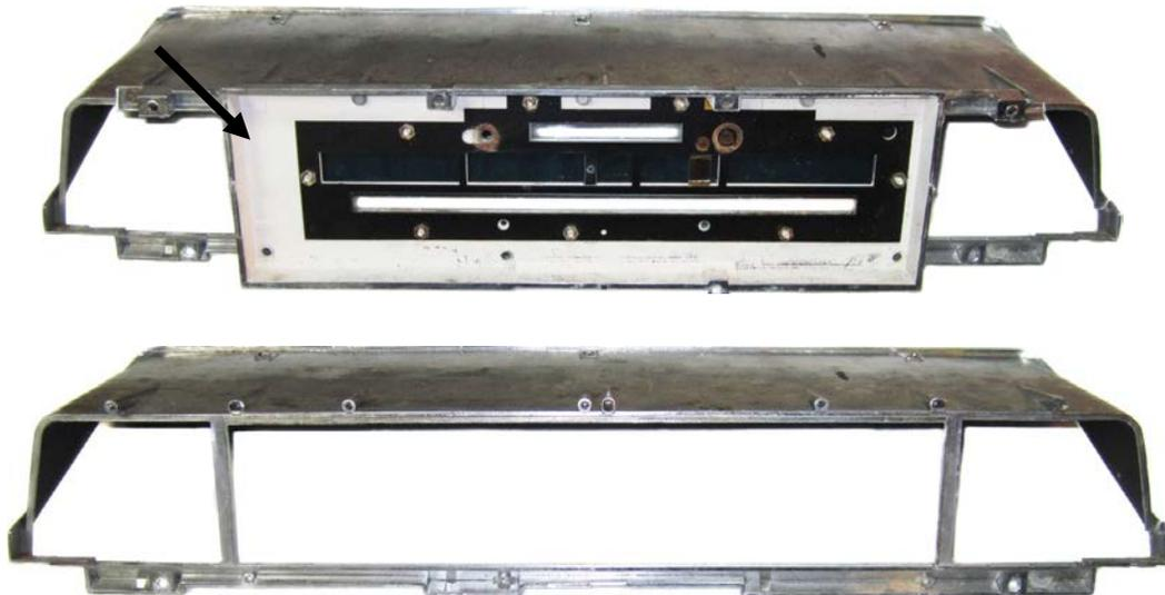
7. Mount the VHX gauge to the gauge trim using the provided three (3) 8-32 X 7/8" screws.
