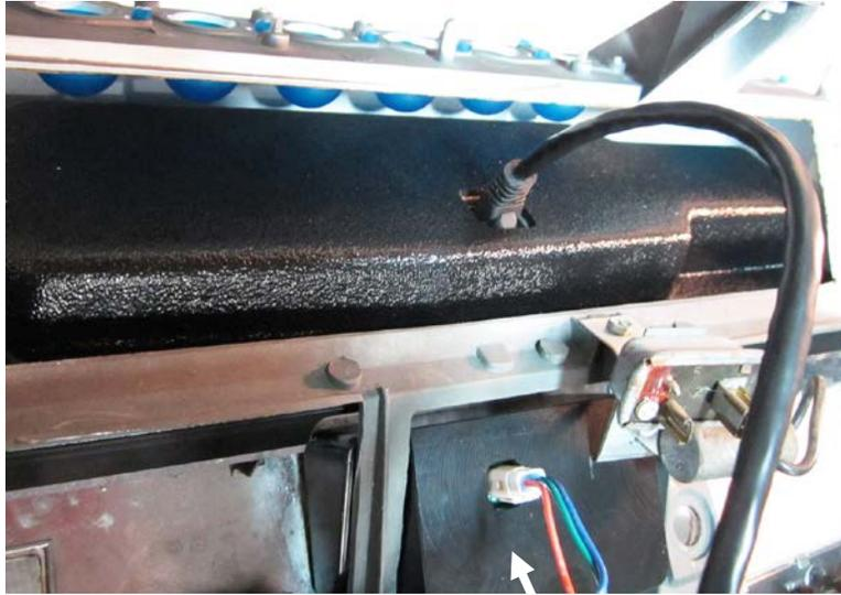
12. Reinstall the lower panel and the dash is now ready to re-install into the vehicle using stock hardware. Take care when routing the CAT5 cable and switch harness to the control box mounting location. Refer to the main manual to complete the VHX installation.
