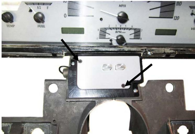
10. Connect the provided switch harness to the back of the VHX switch assembly and refer to the wiring diagram.
