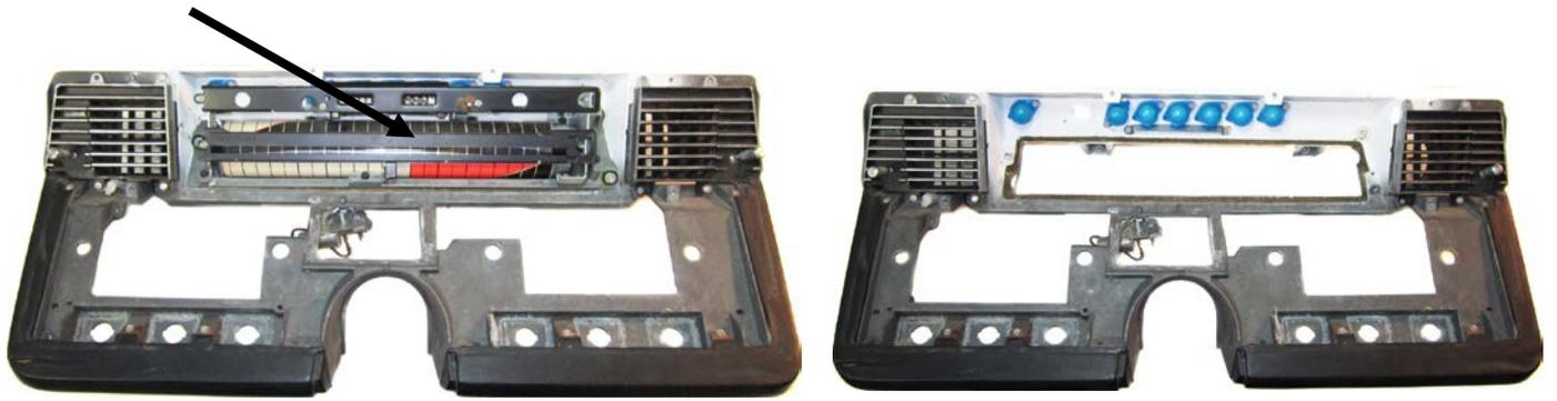
6. Separate the speedometer face from the gauge trim.
