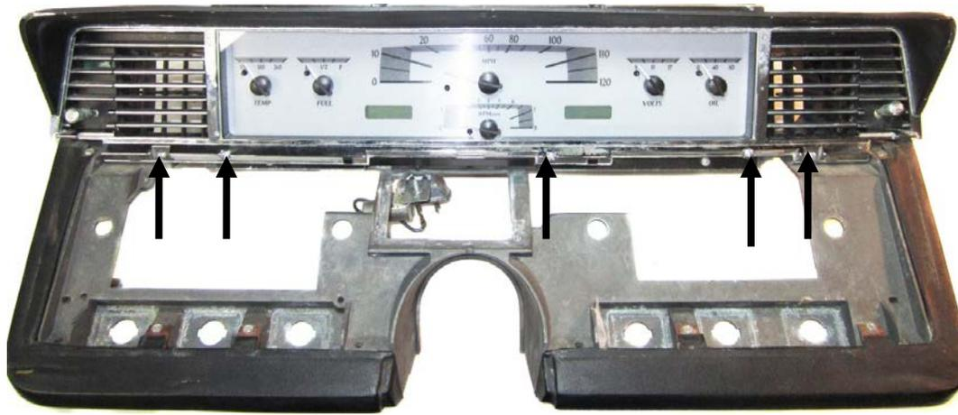
9. Mount the VHX switch assembly to the gauge housing using the provided two (2) 6-32 X 1/4" screws.
