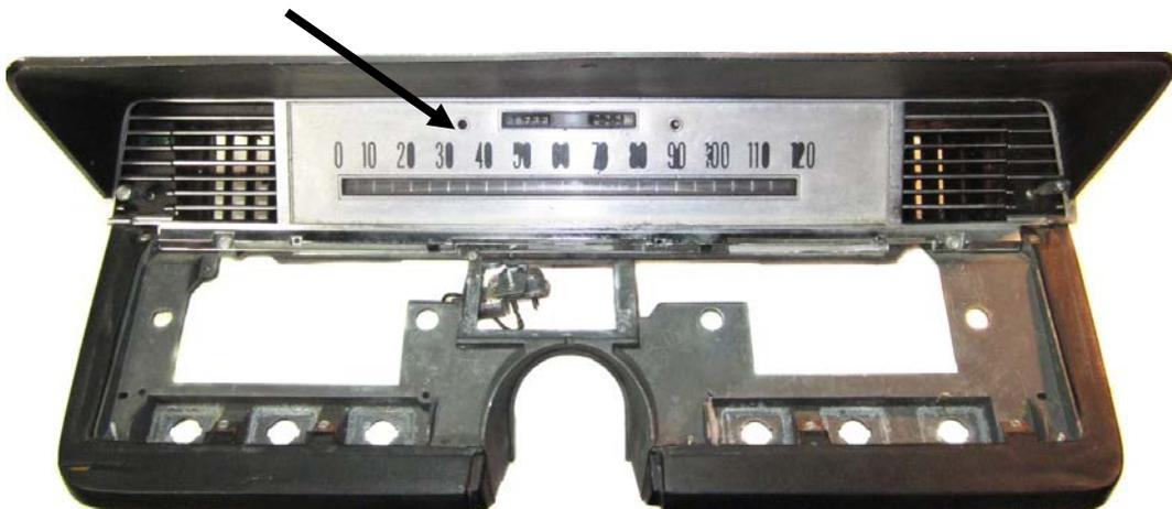
5. Remove the speedometer assembly so you are left with a bare gauge housing. The blue bulb shields can be left in place or removed if desired.
