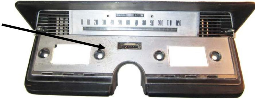
3. Remove the odometer assembly.
