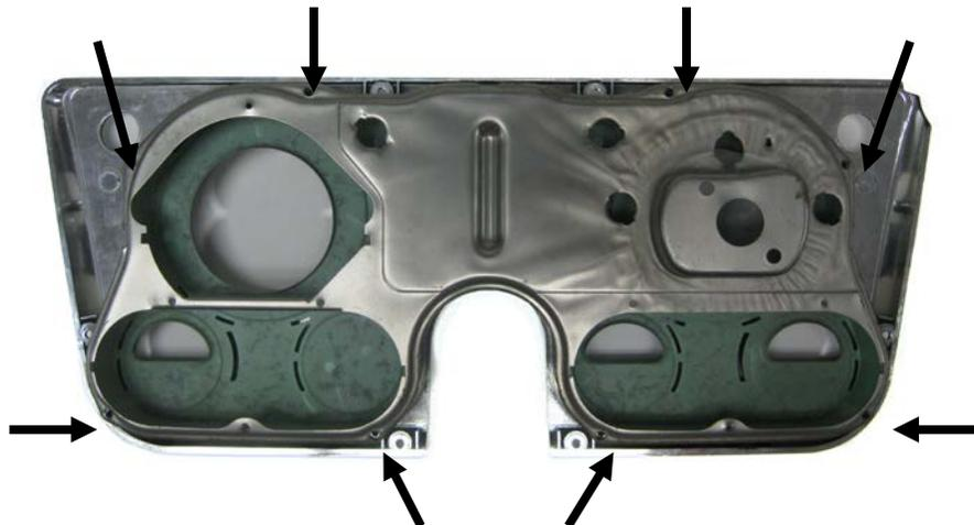
2. Remove the stock gauges, separator plate, and lens from the bezel. The only item to be reused is the original front bezel; the other pieces can be discarded. Now is a good time to clean the bezel and remove any dirt or old lens gasket material.
