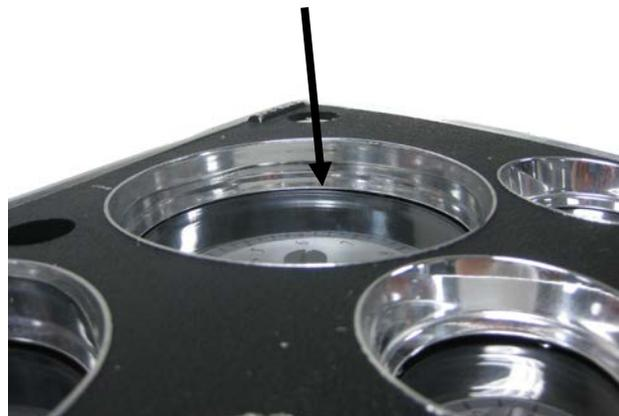
4. Secure the VHX system to the bezel with the eight screws removed from the stock gauges.
