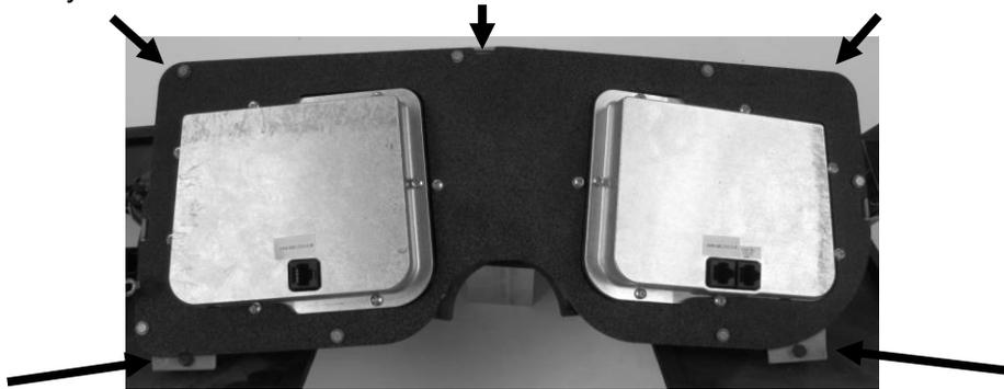
8. Connect the short CAT5 cable between the two gauge housings, then connect the long cable to the system so it can be routed and connected to the control box as the system is re-installed.
