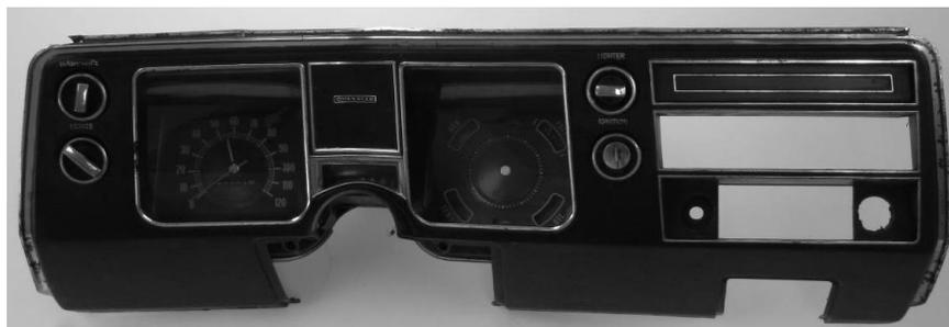
2. Remove the five screws holding the gauges to the bezel as well as the two screws holding ground straps on the back of the system. Save the screws as they will be reused to secure the new VHX system in the steps below.
