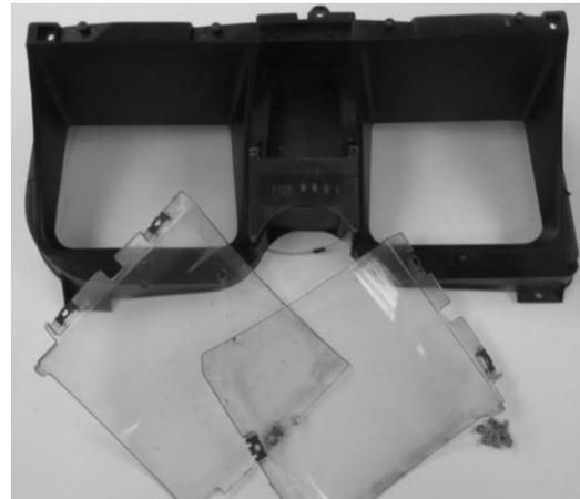
5. This step is optional for automatic transmission bezels only. If you purchased a separate GSS-universal gear kit from Dakota Digital, the gear position can be displayed in the VHX message centers, therefore the stock gear position indicator can be removed.
