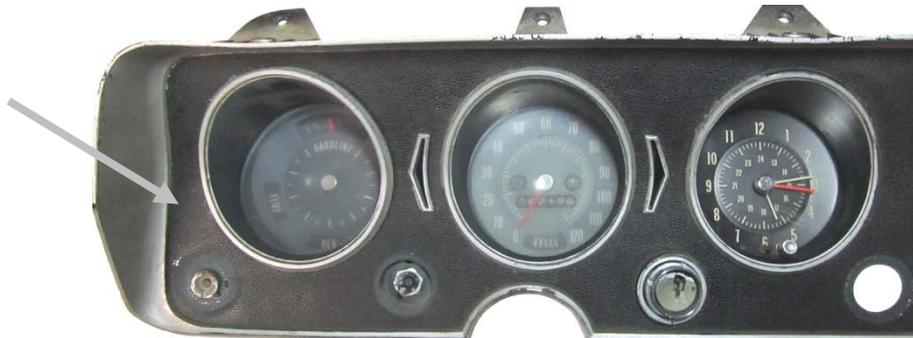
2. Remove the stock gauges from the bezel. The only items to be reused are the original front bezel and the hardware that mounts the gauges; the other gauge pieces can be set aside. Now is a good time to clean or refinish the bezel.
