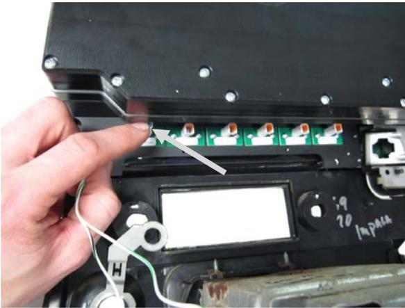
11. If desired the original indicators can be used by connecting the provided harnesses and making the following connections:
