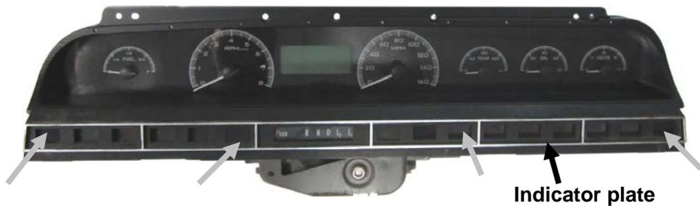
9. Mount the VHX system to the stock bezel using the eight (8) factory screws.
