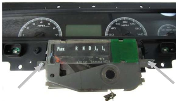
7. There are six (6) small tabs on the back of the indicator plate that will need to be trimmed for proper fit. The locations are shown below.
