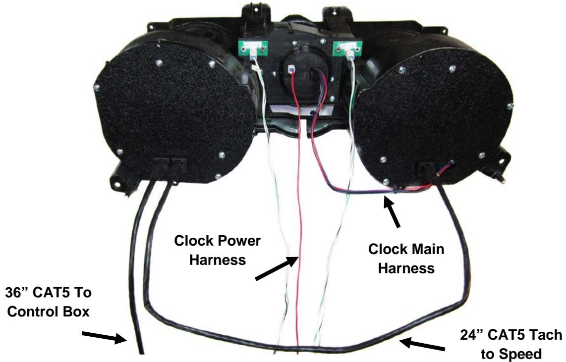
6. Refer to the manuals 650314 and 650462 for wiring instructions to complete the VHX installation.
