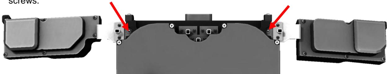
5. Attach the new VHX system to the dash using the original mounting points and hardware.
