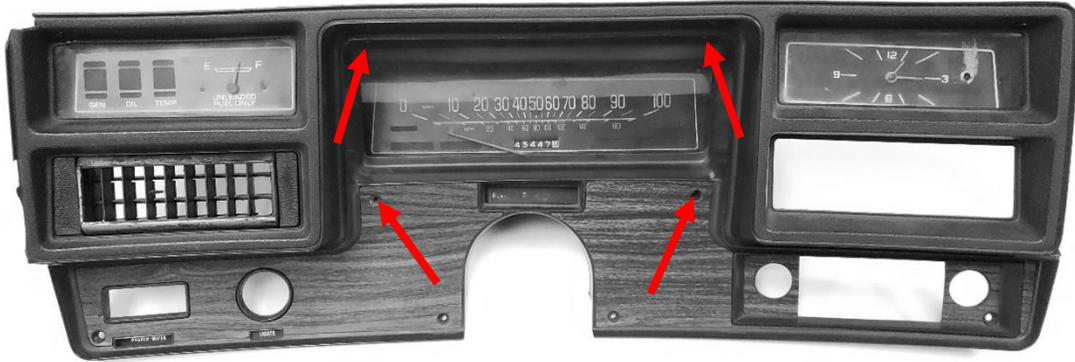
3. Remove the stock lens from the dash. This will require melting the plastic "rivets" fastening the lens to the dash.
