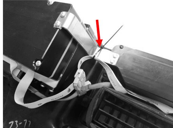
9. When inserting the VHX system and factory bezel into the dash, ensure that the ribbon cables rest in the highlighted locations for the best possible fit:
