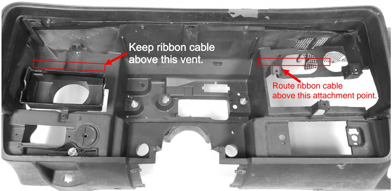
10. Carefully insert the bezel and gauge cluster into the dash, ensuring that the ribbon cables fall into place correctly. Reattach the bezel using the retained original screws.
