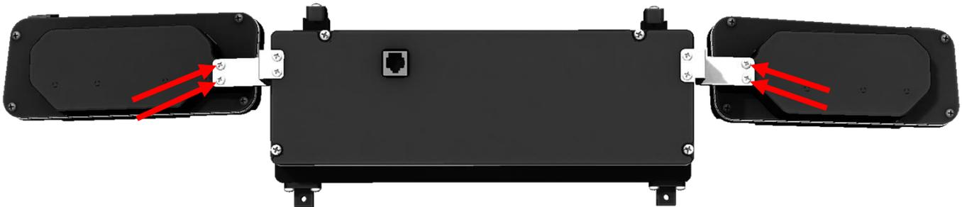
5. Attach the new VHX system to the bezel using the original mounting points and hardware.
