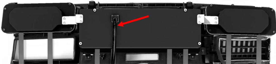
7. Connect the ribbon cables coming out of the main VHX housing to their respective satellite gauges. Each cable is stamped with its corresponding gauge to more easily match them together.
