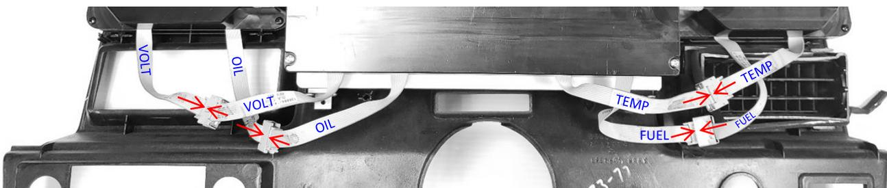
8. Using the two provided cable ties, secure the connected ribbon cables to the positions shown. This will help the ribbon cables to clear the air vent and temperature controls below. Snip any excess cable tie length once attached.
