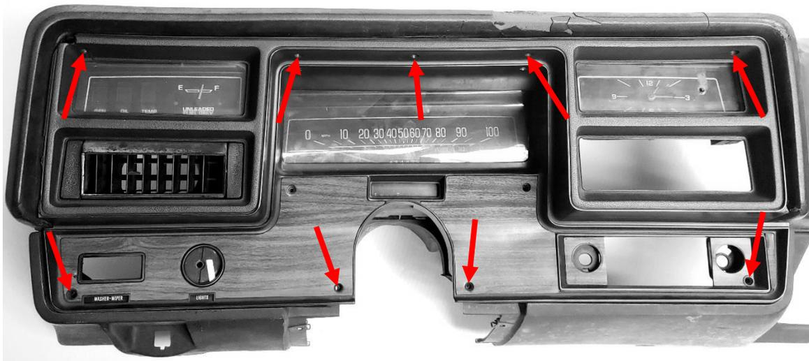
2. Remove the stock gauge cluster from the bezel. The gauge cluster is held in place by four screws in the center of the bezel. Save the screws obtained as they will be re-used to secure the new VHX system.
