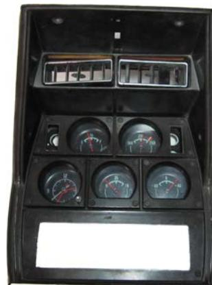
2. Remove the stock gauge assembly from the center gauge bezel; the only items to be reused are the front bezel and the gauge mounting hardware. Now is a good time to clean or refinish the bezel.
