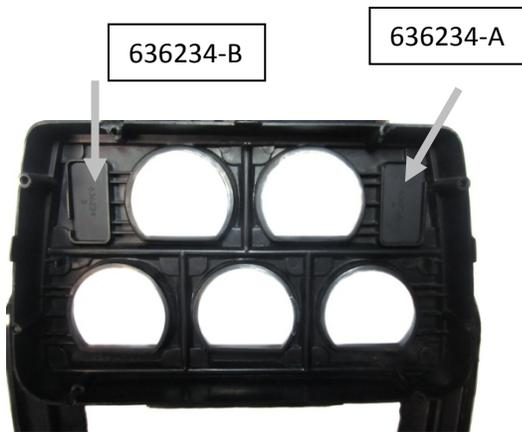
3. Peel the paper off the two block-off lenses needed (636234-A and 636234-B) and place them shiny side down in the two rectangular openings. Use silicone to hold them in place and avoid handling until the silicone has cured.
