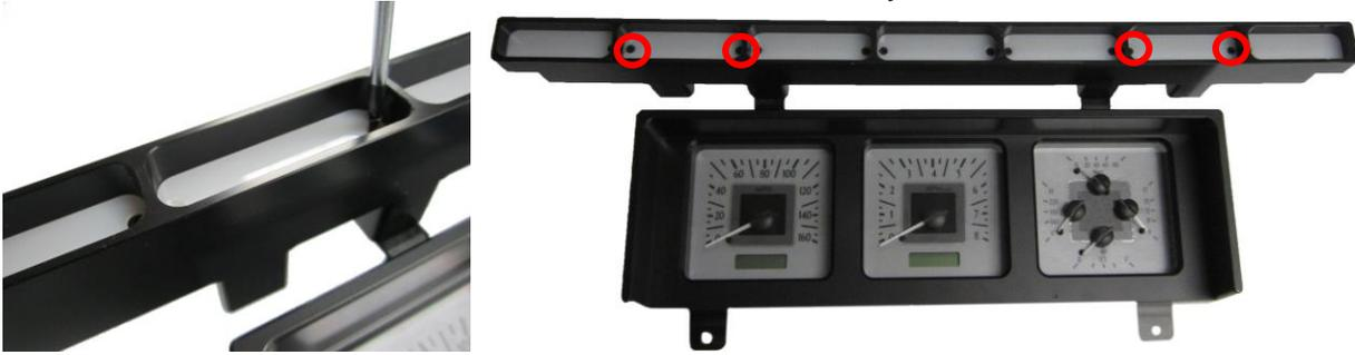
5. Take the bezel and test fit it onto the VHX display. If the indicator panel doesn't fit into your bezel properly, loosen the eight Philips screws and adjust as needed. Once adjusted, lightly tighten the Philips screws to prevent further adjustment.
