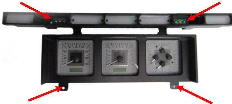
7. Re-install the two white acrylic lenses and four Philips mounting screws.
