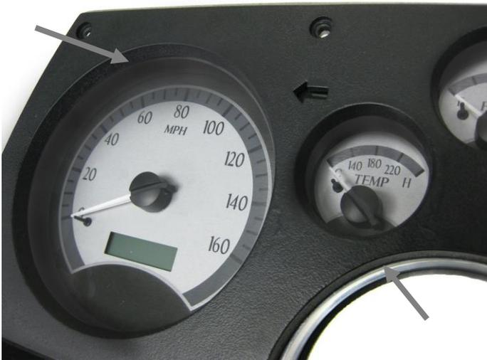
4b. The VHX system should fit tight and the lens should sit flush with the bezel.
