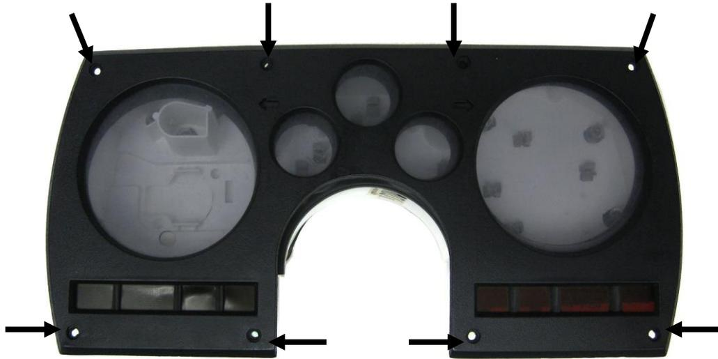
2. Remove the stock gauges, light indicators, and lens from the bezel. The only item to be reused is the original front bezel; the other pieces can be discarded. Now is a good time to clean the bezel.
