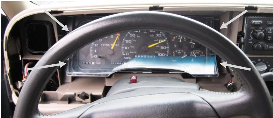
2. At your own discretion, carefully cut directly above the stock gauge connector to allow more length on the harness side for the required cut and splice wiring. Also, the harness connector will need to be pushed out of the way to clear the VHX cluster; opening up the inner structure will allow space needed for clearance, otherwise the connector will need to be removed.
