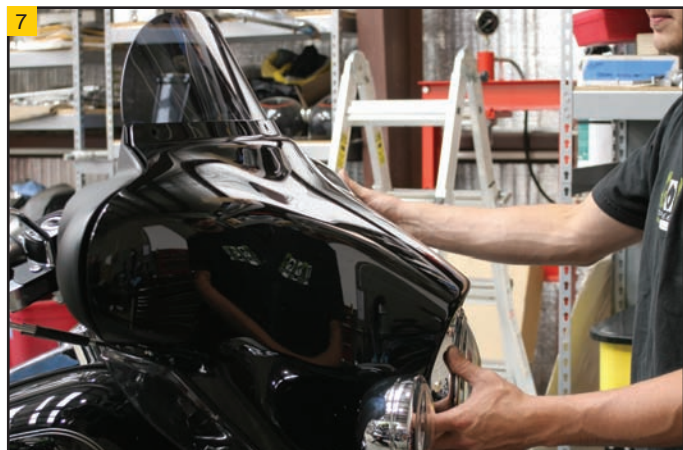
Plug the headlight back into the wiring harness, and reassemble the fairing.
