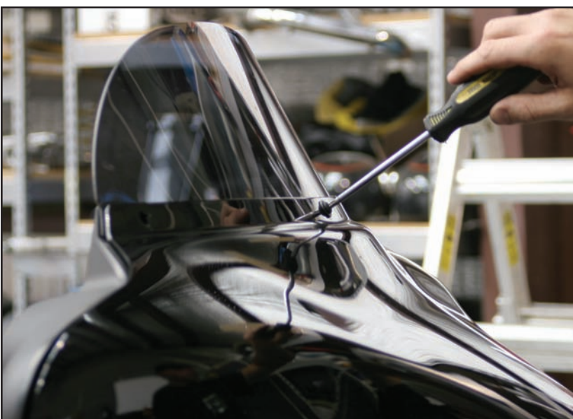
Finally, put the screws back in the outer fairing, and then crank up that radio and go cruising.
