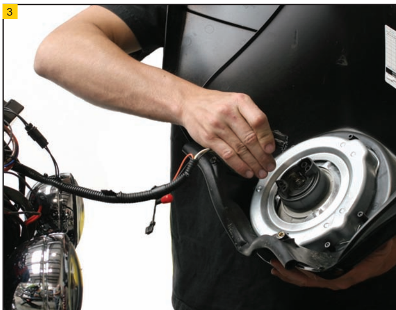
3 Disconnect the headlight, and set the outer fairing aside.
