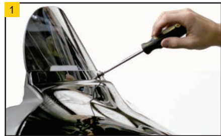
1 Remove the screws holding the outer fairing in place.
