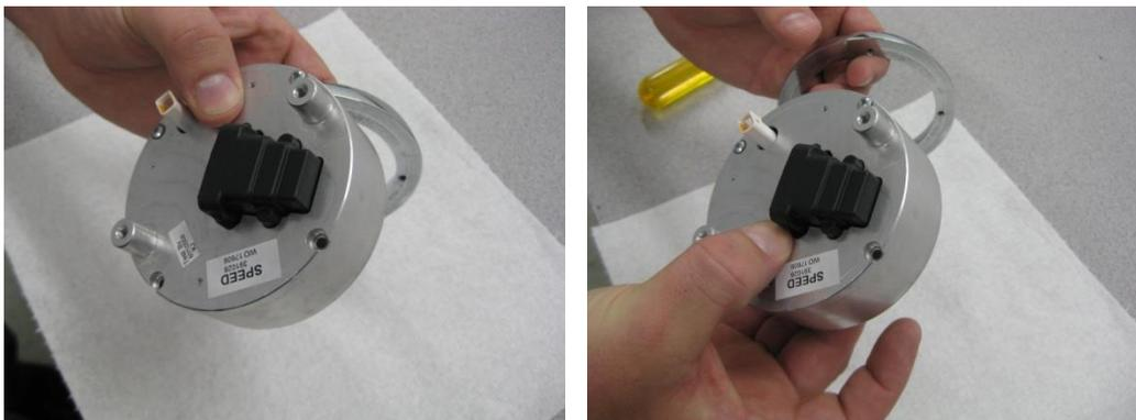
Locate a large black bezel and four of the 4-40 x 1.25" screws. While holding the gauge housing and lens, install one of the screws from the back of the housing and up through the lens, hold the screw in place with your finger. Carefully align this screw with one of the holes in the bezel to get started.
