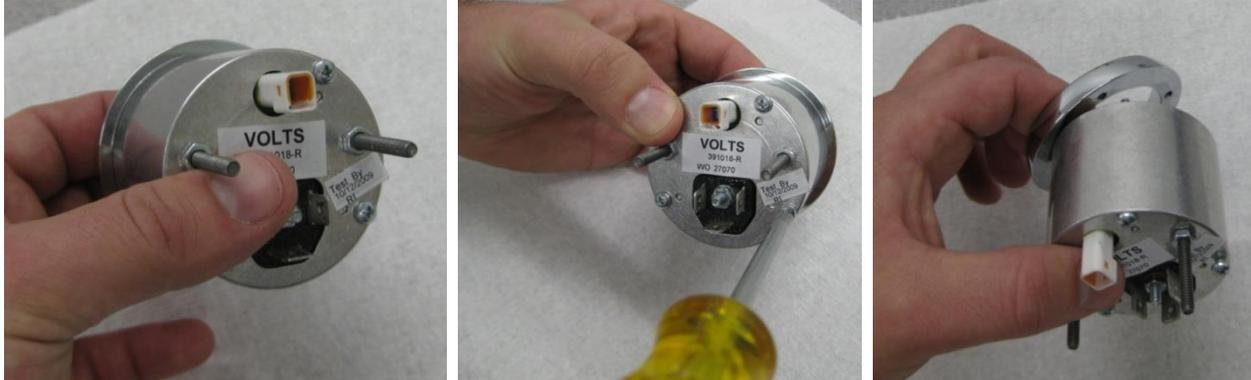
Locate a small black bezel and three of the 4-40 x 1.75" screws. While holding the gauge housing and lens, install one of the screws from the back of the housing through the lens. Hold the screw in place with your finger; carefully align this screw with one of the holes in the bezel to get started, using caution to not scratch the lens.
