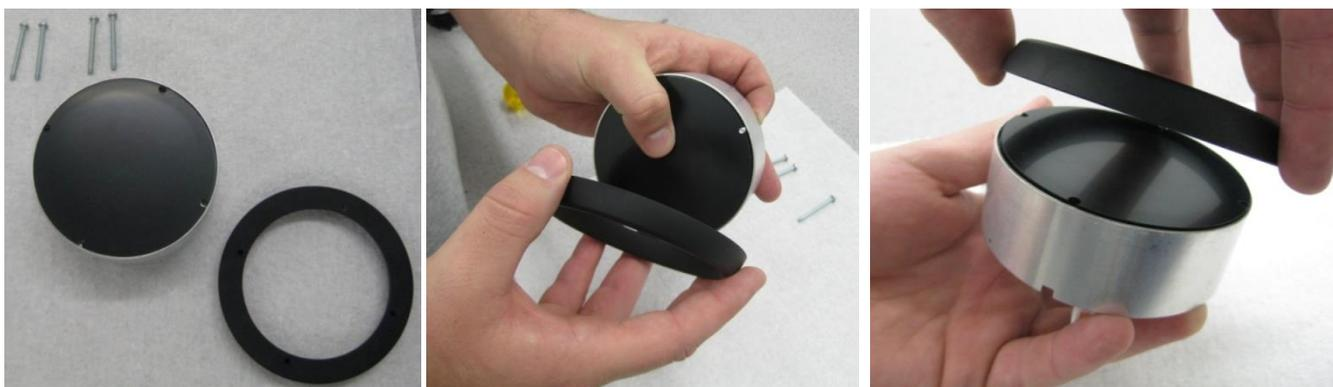
Start one screw a couple turns, do not fully tighten. Use care when aligning the bezel to avoid scratching the lens, pivoting off the started screw as needed, then start the remaining three screws. Tighten up the remaining screws in a criss-cross pattern, approximately 5.5 in-lbs of torque. DO NOT over tighten!
