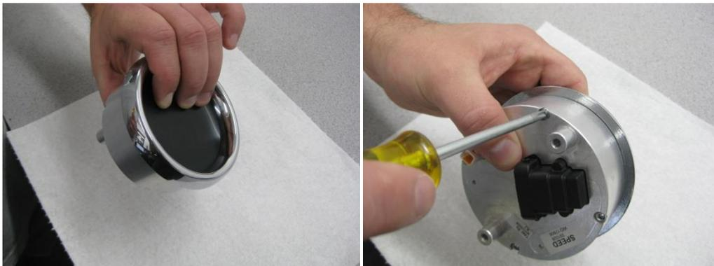
Once the four screws are removed, hold the lens and gauge housing so the lens does not fall out or move. Carefully remove the chrome bezel.
