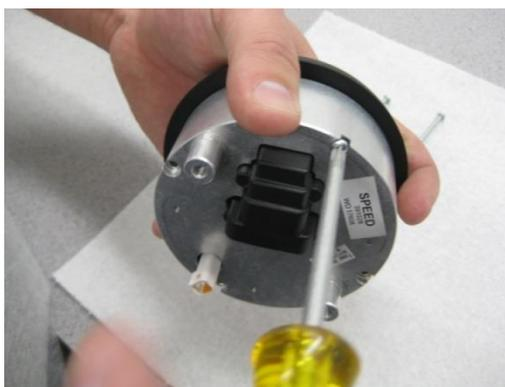
Bezel install is complete, re-install gauge and repeat the steps for the second large gauge.
