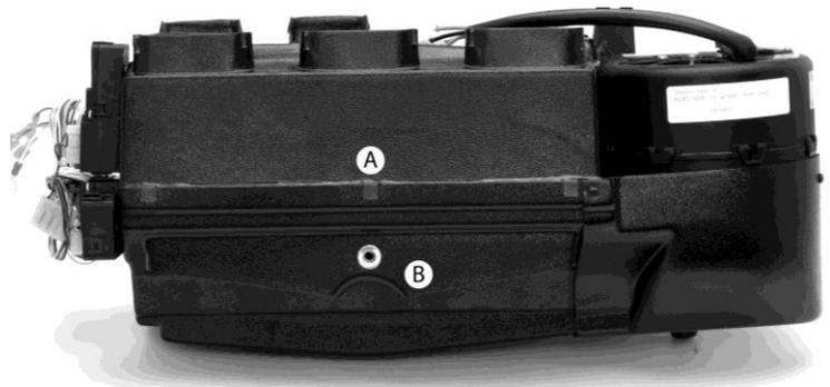
**Figure 6:** MINI temp sensor placement. A) vent sensor B) floor sensor
