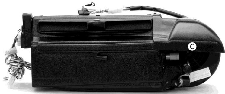
**Figure 7:** MINI Cabin temp sensor placement. (point C)
