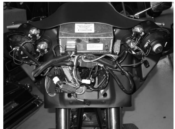
Road Glide with outer fairing removed
