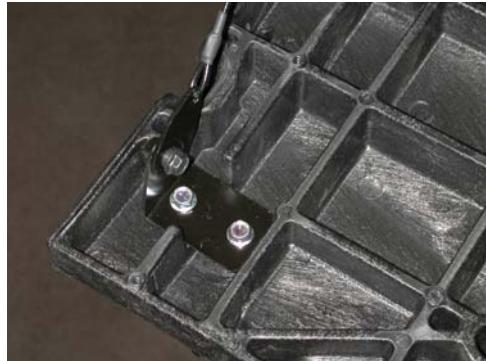
3. Remove the tailgate strap from the side you are working on. Remove the (2) 10MM bolts holding the strap bracket to the latch. Use the same bracket and bolts to install the new latch, reinstall the strap.
