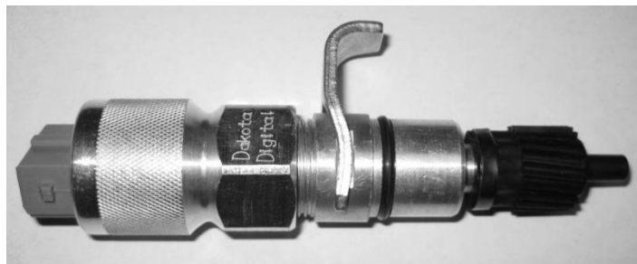
New sensor installed on adaptor
