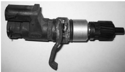
Original speed sensor removed from transmission
